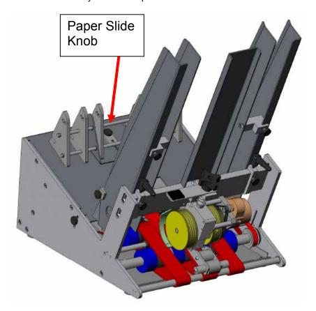
Figure III-9 Shrouded Separator
