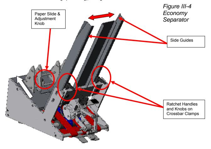
6. Insert the setup piece between the separator wheels and the blue nip rollers. While moving the setup piece back and forth beneath the separator wheel, turn the separator adjustment knob counter-clockwise (CCW) until resistance is felt from the separator wheels (see later discussion on fine-tuning of the separator wheel), see figure III-5.
