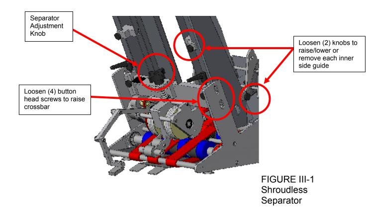
2. Raise both separator wheels by turning the adjustment knob atop separator assembly in a clockwise direction, see figure III-1. (Shroudless separator shown)
